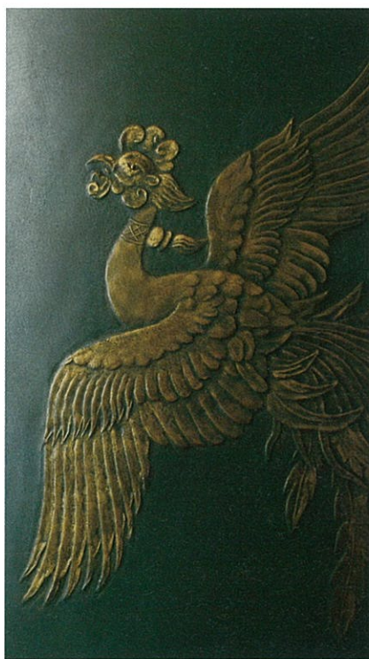
Interior wall of a temple bell's outer mold (overleaf). A well-made mold will produce detailed relief figures and inscriptions, for which careful finishing is essential. Other fine craftsmanship can be seen in the magnificent bell at Zuisen-ji and in dragon-shaped suspension braces.
